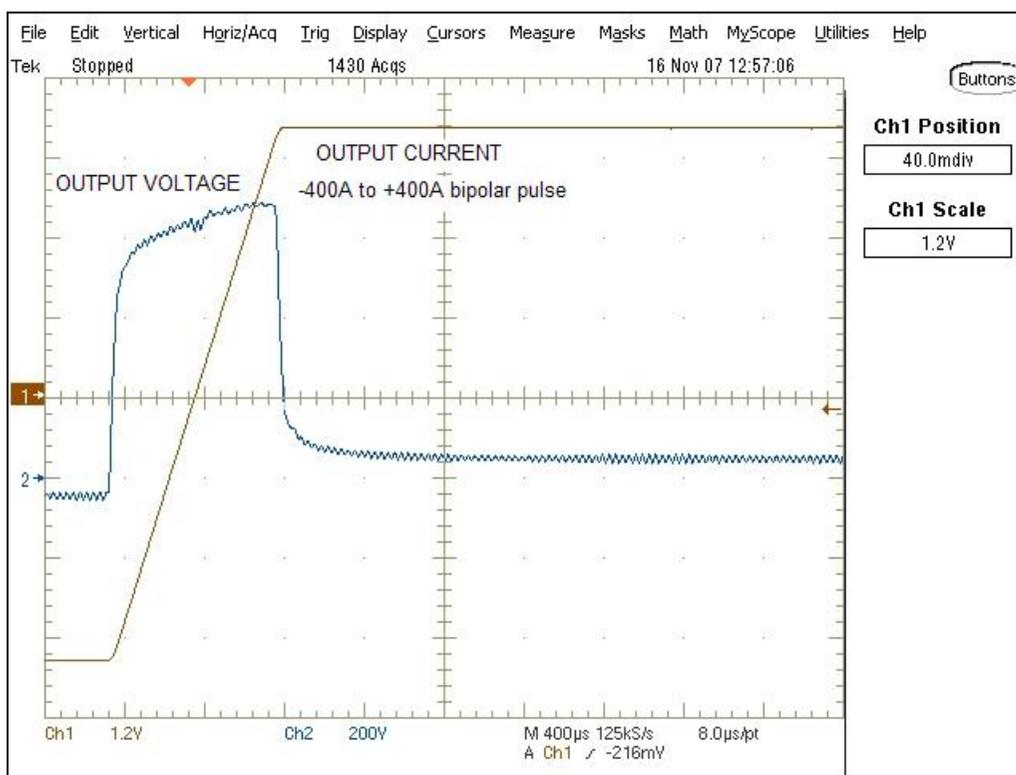
Amplifier output current and voltage waveforms to 580 µH gradient coil
